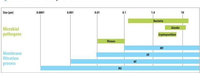
Figure 2.2 Membrane filtration pore sizes
