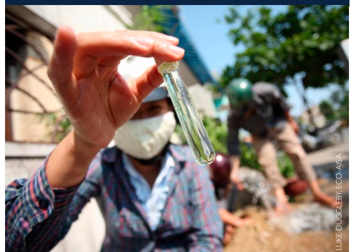
Staff from the Da Nang Water Supply Company takes a sample of water to test for chlorine residuals in the pipe network.
