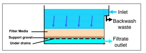
Properly designed and operated filters can remove a wide range of potential contaminants and are thus a key part of the water purification process. They are effective in removing suspended & particulate matter including associated substances such as:
